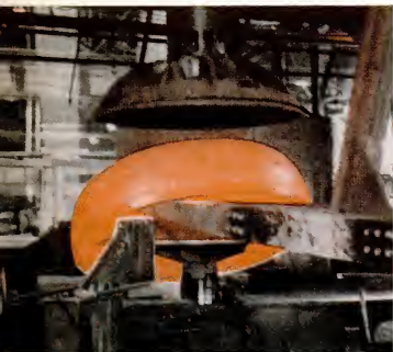
NUDGED ONTO THE FORM , the workpiece is centered by guides as the peel withdraws.
